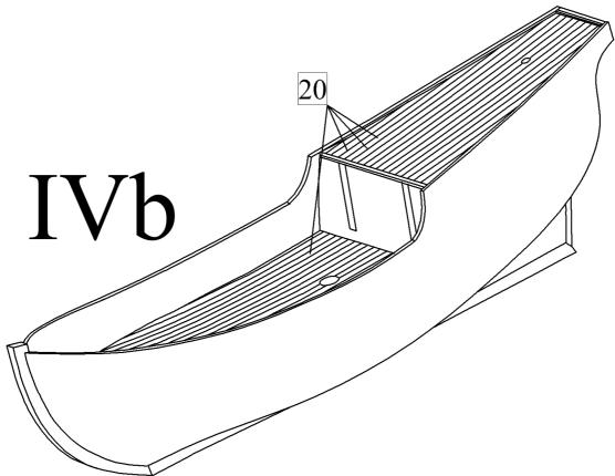
c) Make hatches on the deck. First glue frames of the hatches from parts 21 and 128 and 129. Then glue this frames to the deck. Then plank the hatches by strips 22. Finally glue parts 23-25 to the hatches.
