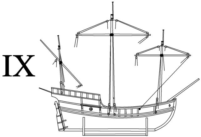
a) First tie yards to the masts. Then run the ropes for raising and lowering of the yards through holes in the masts and then tie them to the blocks 117 and 79. Finally tie also the rest of ropes to the yards.
