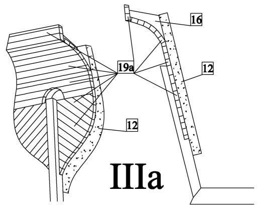
b) Plank a hull of the ship by strips 19b. Before planking bend the strips into required shape (A procedure of the strip bending is described in a start of this document). Start the planking from stem with strips on upper edge of the hull. Then continue with planking to the stern.
