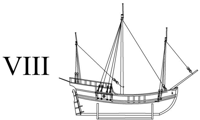
a) First glue masts to the hull and then tie also shrouds to the masts.
