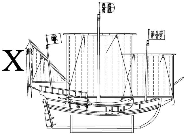
a) Make a sail 118-120. First draw by pencil contours of the sail on the. To the border of the sails add about 10mm for fell. By the pencil draw on the cloth also seams which divided the sail into simple segments. Then scissor the sail with fells and sewn it like it is shown below.
