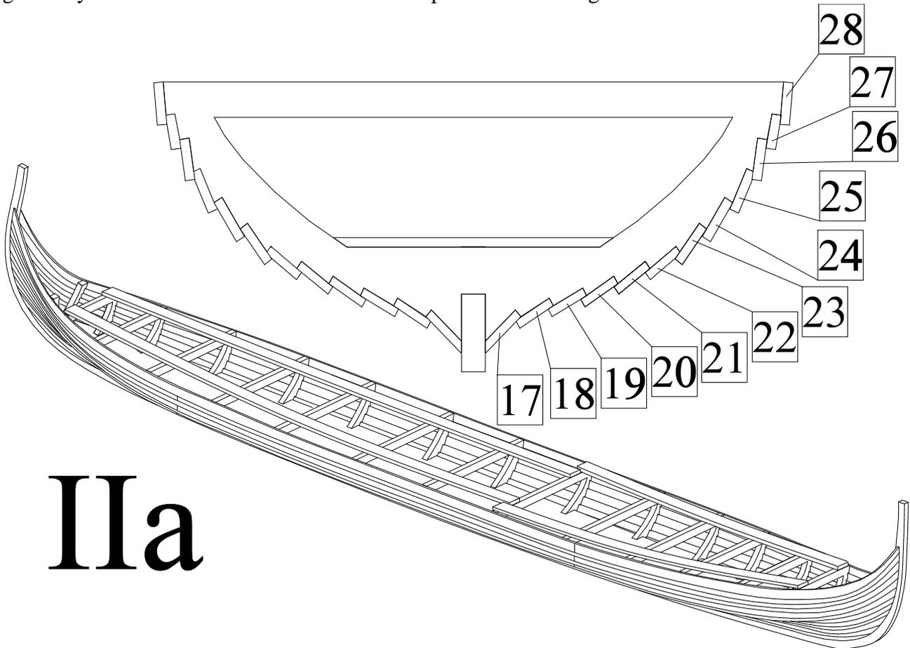
b) Cut off the parts of ribs 1-13, which overlap the deck. Attention! Ribs 15 and 16 leave in the original state.
